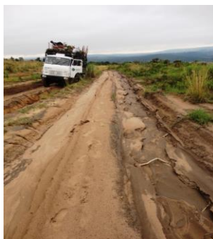
Photo 8 : heavy truck in difficulty rolling due to severe ruts to Case Barnier.
